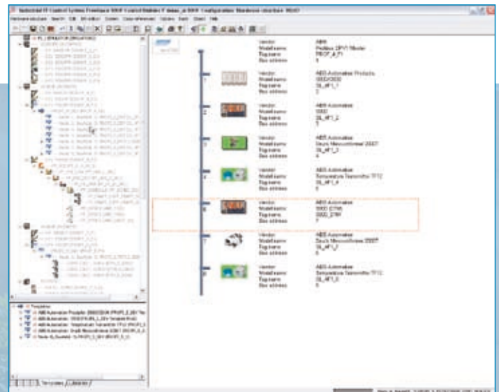
Configuration of the fieldbus line (PROFIBUS)
